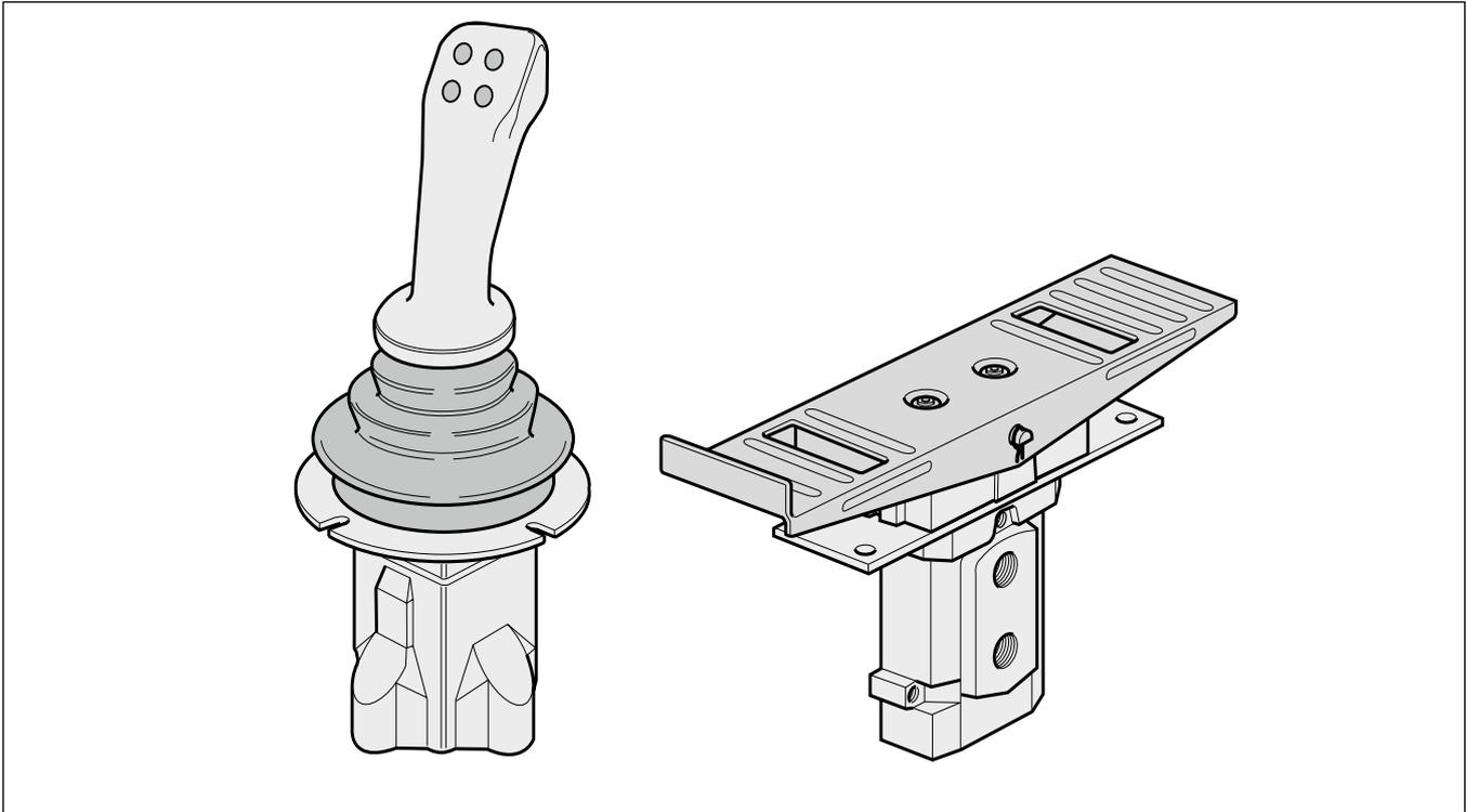
The PCL4 is a stackable hydraulic control-pressure valve intended for the proportional, hydraulic remote control of directional valves, pumps with variable displacement, positioning cylinders, etc. It can be obtained with a co-ordinate lever (joystick), linear lever or foot pedal as the activating device.
